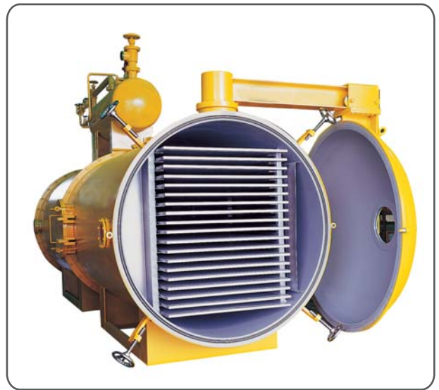
真空乾燥設備(2) Vacuum Freeze-Drying Unit (2)
